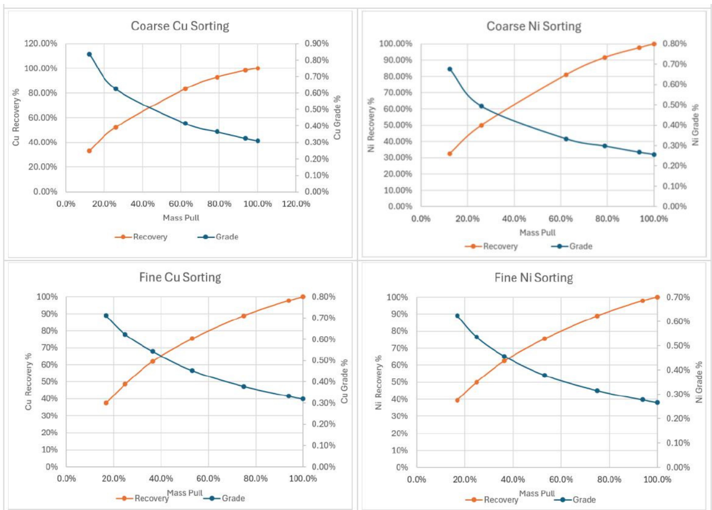
Figure 13-1 Coarse and fine copper and nickel recovery versus mass pull curves
