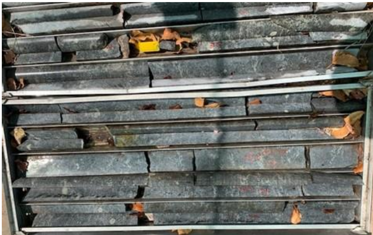
Figure 12-3: DSLK278 – Dikgaka Gabbro
