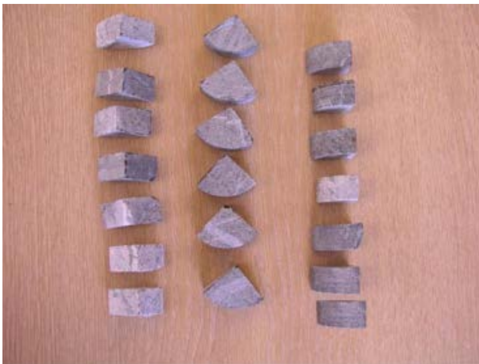
Figure 5 – Orientations of Pieces for Breakage (Cut Core Method)
