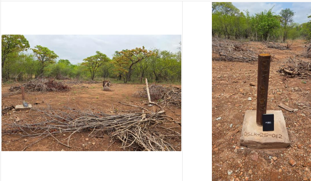
Figure 12-10 Twin drilled collars (left) and infill drillhole collar (right)
