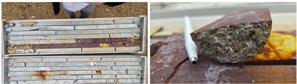
Figure 12-9 Oxidised TMNC core at Selkirk
